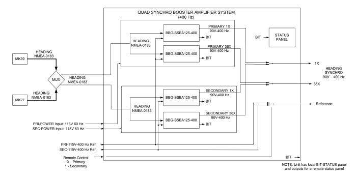
The BBG-RSSS-90-400-1 operates on 115 Volt, 60 Hz AC power to convert serial inputs into high power synchro outputs. The RSSS accepts serial data in RS-232, RS-422, RS-423, RS-485, or MIL-STD-188C protocols. Serial baud rates are switch selectable at: 2400, 4800, 9600, 19,200, and 38,400 bits per second. Default serial input is 4800, 8 bits, no parity, and one stop bit (4800, 8, N, 1).
