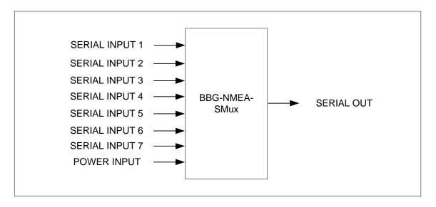
The BBG-NMEA-SMux operates on +24 VDC input power and performs serial combining of up to seven (7) NMEA-0183 serial inputs into one NMEA-0183 serial output. Input and output baud rates are switch selectable and status LEDs show input activity and system status
